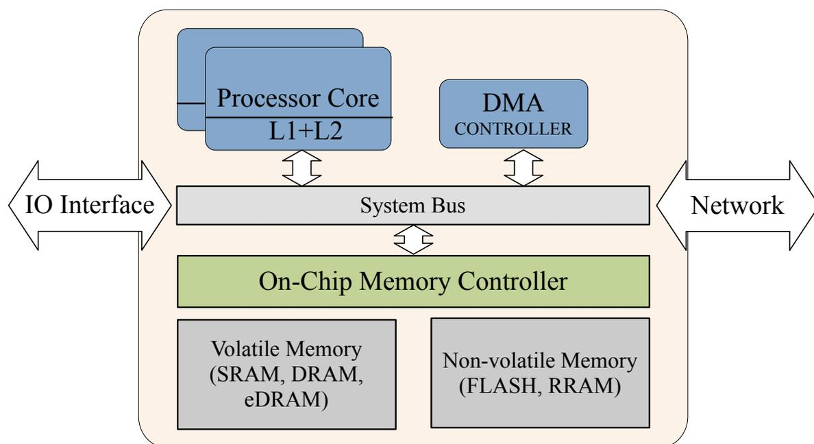
**Figure 4.** Illustrative example of a mobile IoT system.
