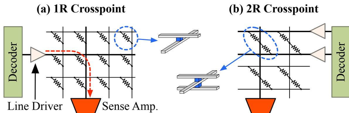
**Figure 5.** Illustrative examples of 1R (a) and 2R (b) crosspoint arrays.
