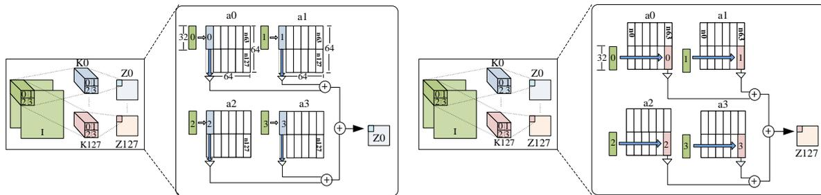
**Figure 13.** Distribution of a convolution layer to the crosspoint arrays: input feature map is convolved with kernel  $K_0$ , and input feature map is convolved with kernel  $K_{127}$ .
