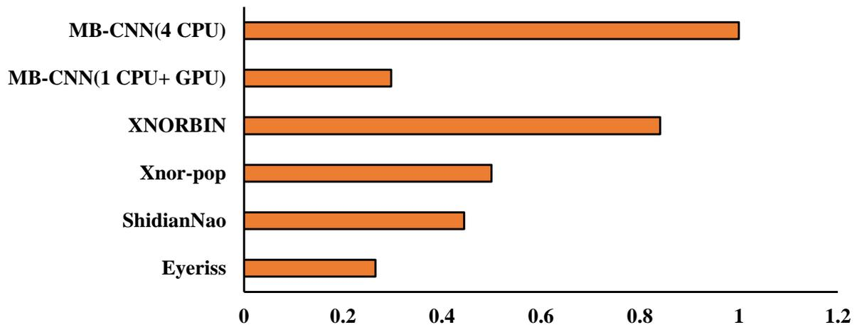
Figure 19. System Energy per frame for different state-of-the-art accelerators relative to MB-CNN.
