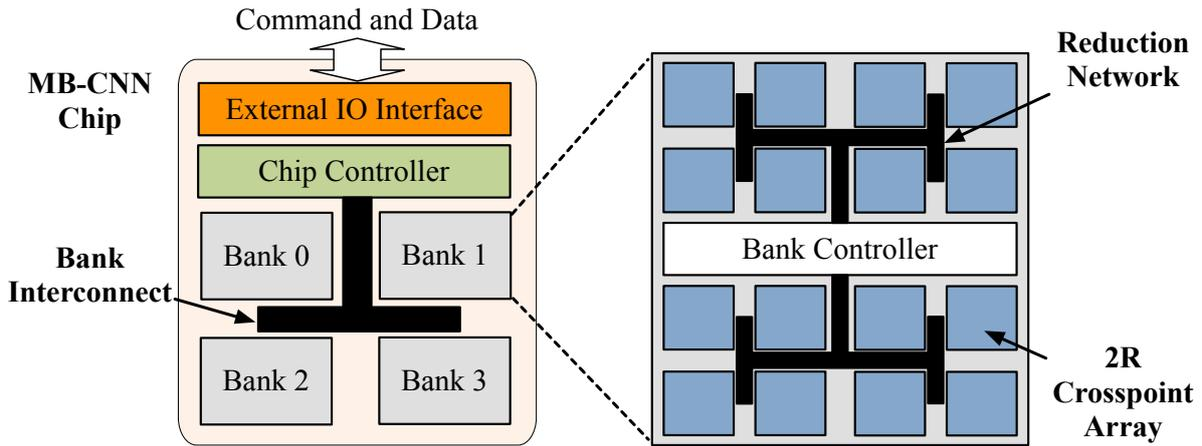
Figure 10. The proposed hierarchical organization for the accelerator.
