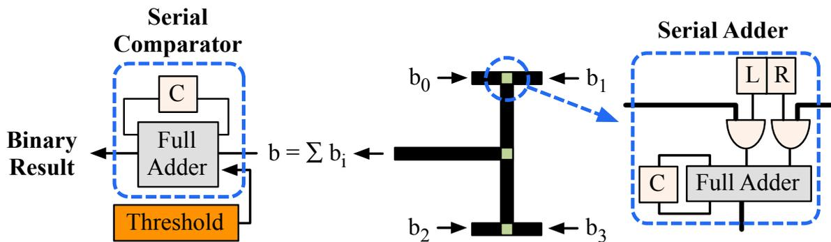
Figure 11. Merging bit-counts into a single result inside a bank.
