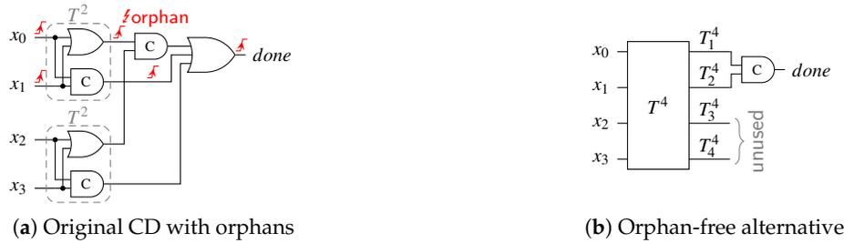
Figure 15. 2-of-4 completion detectors.
