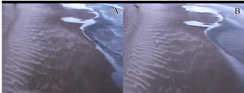
Figure 3. Example of a snapshot (A) and timex image (B). Streamers and waves are visible in the snapshot, but they are blurred out in the timex image. The images were taken on 25-09-2012 around 6.00 h (GMT). The hourly mean wind velocity U was 8 m/s and the wind direction \theta was 97^\circ . \theta = 0^\circ is cross-shore from the west, \theta = -90^\circ is the alongshore wind coming from the north, and \theta = 90^\circ is alongshore from the south.
