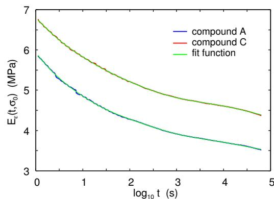
**Figure 6.** Dependence of the (nonlinear) strain relaxation modulus  $E_\epsilon(t, \sigma_0) = \sigma(t)/\epsilon(t)$  on the time obtained from the data in Figure 5. The red and blue lines are the measurement results for compounds C and A, respectively, and the green lines the fitted curves using the fit function (10).
