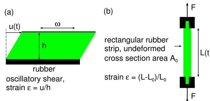
**Figure 1.** (a) Method used to measure the shear modulus  $G(\omega, \epsilon_0)$ . The upper plate oscillates in a plane with frequency  $\omega$  and strain amplitude  $\epsilon_0$ . (b) Set-up used for measuring the strain relaxation modulus  $E_\epsilon(t, \sigma_0)$ . The force  $F$  is applied at time  $t = 0$  and the length of the rubber strip is measured as a function of time.
