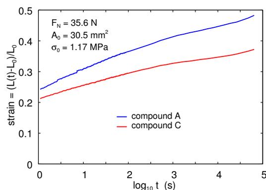
**Figure 5.** The dependency of the strain on time. At time  $t = 0$ , a force  $F = 35.6$  N is applied to a rubber strip with the (undeformed) cross section  $A_0 = 30.5$  mm<sup>2</sup>. The red and blue lines are the measurement results for compounds C and A, respectively.
