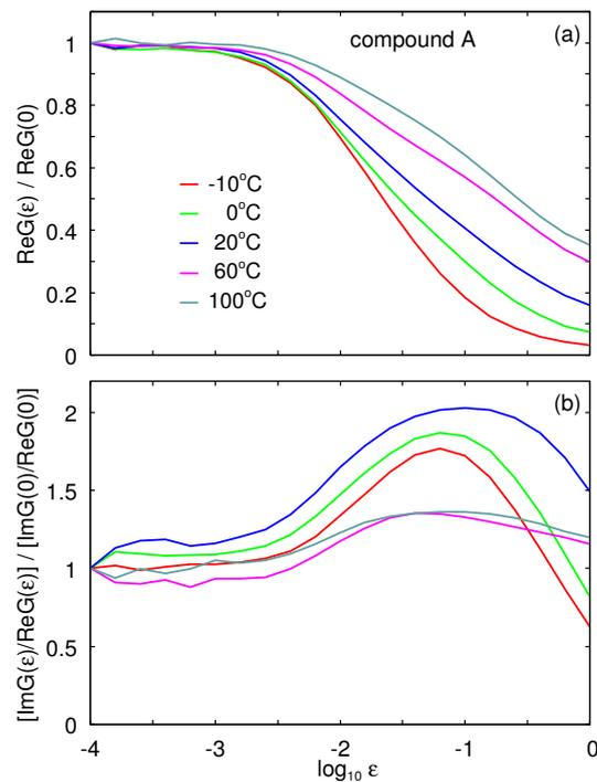
**Figure 4.** (a) The ratio of the real part of the shear modulus  $G(\epsilon)$  for the strain  $\epsilon$  and for vanishing strain (or actually  $\epsilon = 0.0001$ ). (b) The ratio between  $\text{Im}G(\epsilon)/\text{Re}G(\epsilon)$  for the strain  $\epsilon$  and the same quantity for vanishing strain. Results are shown for the temperatures  $T = -10, 0, 20, 60$  and  $100^\circ\text{C}$ . The shear modulus is measured in oscillatory mode at the frequency  $f = 10$  Hz.
