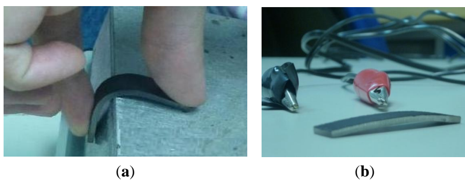
Figure 5. Probe coated with conductive ink in its temporary shape (bended) and after its original shape recovery through heating (almost linear). Infrared thermographs showing the heating process and the related shape recovery, as well as the remarkable homogeneous temperature achieved.
