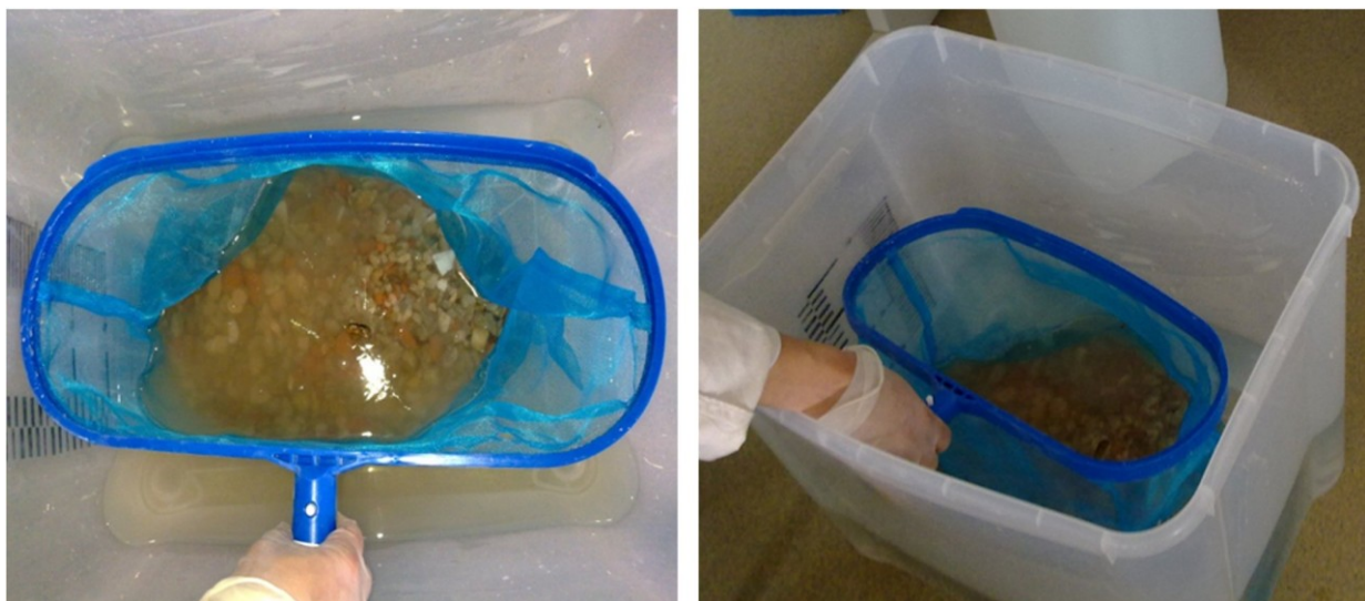
Figure 2. Pre-saturation of recycled aggregate prior to the addition in the concrete batch.
