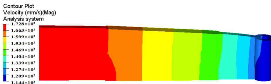
Figure 10. Velocity distribution in the extruded profile for the first modification scheme.
