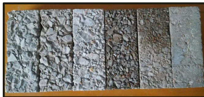
Figure 1. Concrete surfaces with different roughness.
