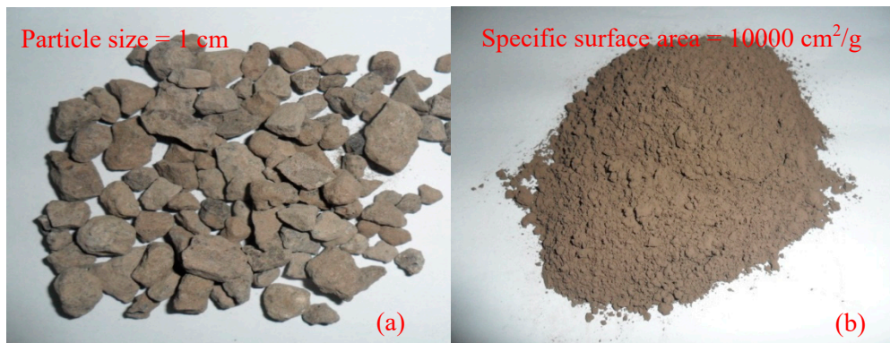
Figure 1. Appearance of BOFS before grinding (a) and after grinding (b).
