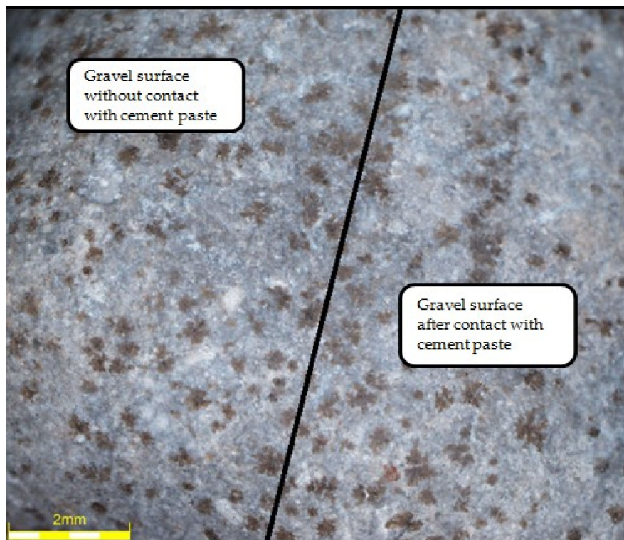
Figure 19. Gravel after thermo-mechanical treatment.
