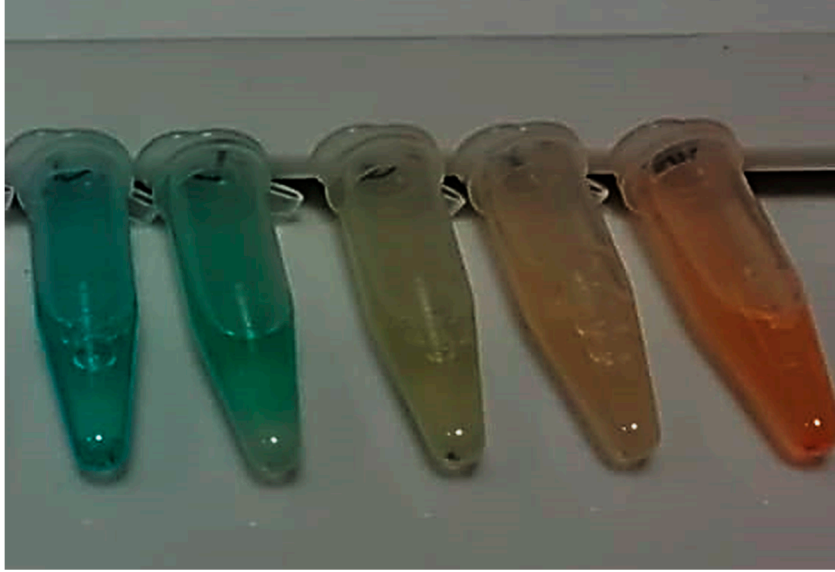
Figure S4. Stability of Dz in Triton X114 at different pH. From left to right: pH 3,5,6,7,8.
