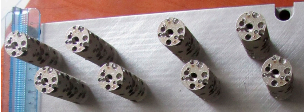
Figure 12. Cylindrical random foams manufactured by means of LPBF.
