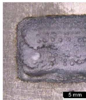
Figure 9. Detail of surface irregularities of the first layer for 75% OR.
