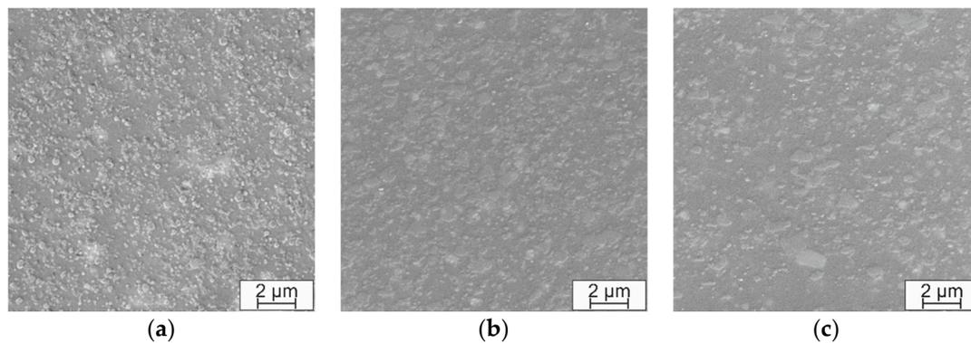
**Figure 3.** SEM images of AMCs produced by means of high-energy ball milling, hot isostatic pressing and extrusion in the T4 condition; matrix alloy AA2017; reinforced with SiC particles: (a) 15 vol %  $\beta$ -phase with size  $< 0.2 \mu\text{m}$ ; (b) 15 vol %  $\alpha$ -phase with size  $< 1 \mu\text{m}$ ; and (c) 10 vol %  $\alpha$ -phase with size  $< 1 \mu\text{m}$ .
