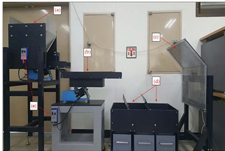
Figure 3. Photograph of the induction electrostatic separation unit: (a) Feeder, (b) positive electrode, (c) negative electrode, (d) splitter and bins, and (e) feed rate controller.
