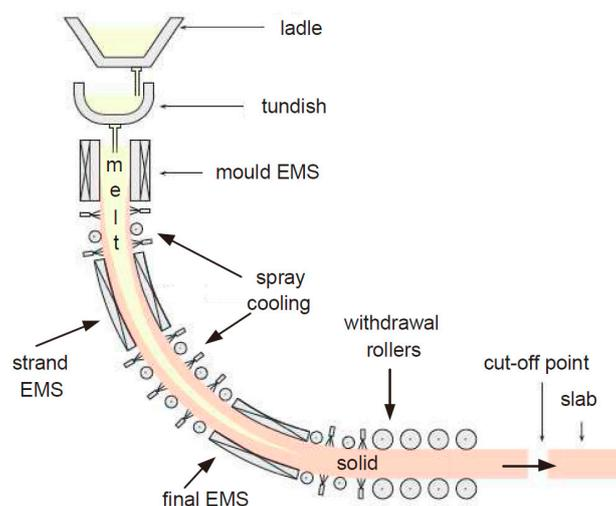
**Figure 1.** Schematic for the continuous casting of steel.
