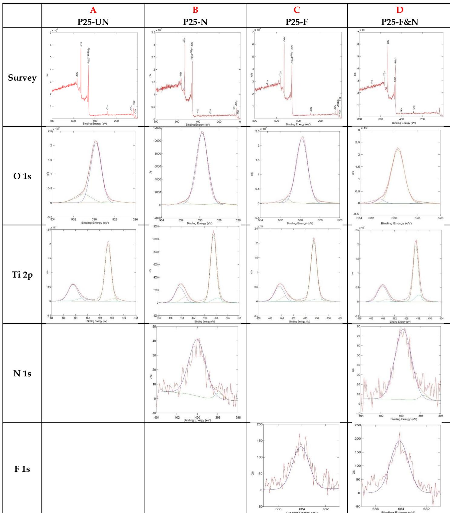
**Figure S2.** XPS spectra of undoped and doped samples and high-resolution analysis in the O 1s, Ti 2p, N 1s, and F 1s binding energy regions.
