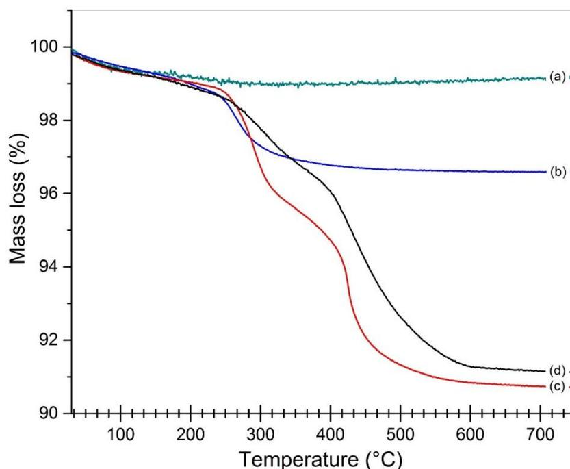
**Figure S1.** TGA profiles showing the weight loss versus the temperature of P25-UN (a); P25-N-Att (b); P25-F-Att (c); and P25-N&F-Att (d).
