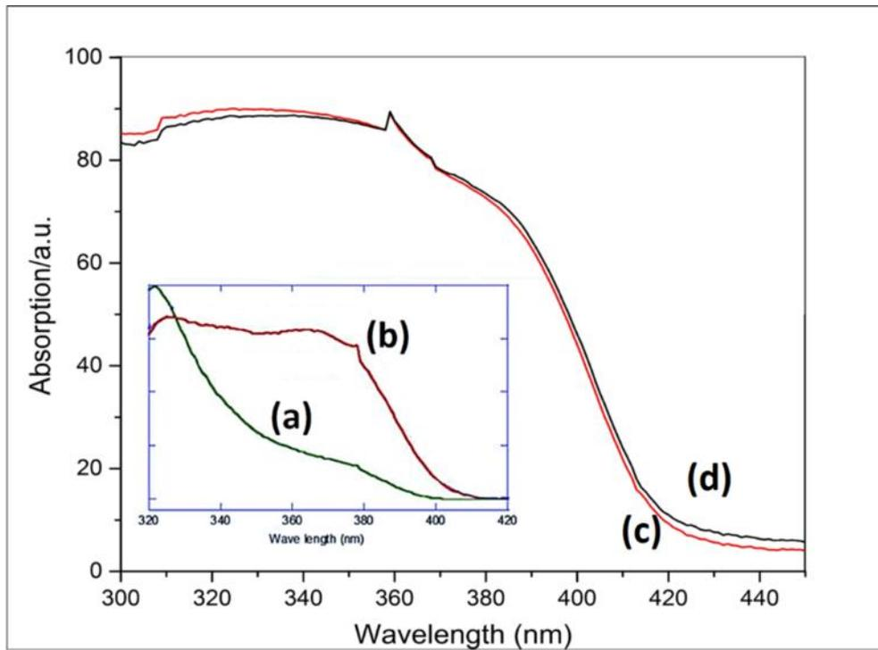
**Figure S4.** UV-Vis-RS spectra of various samples. P25-UN (a) and P25-N-HT (b) (these were separated in the inset for more clarity), P25-F-HT (c) and P25-N&F-HT (d).
