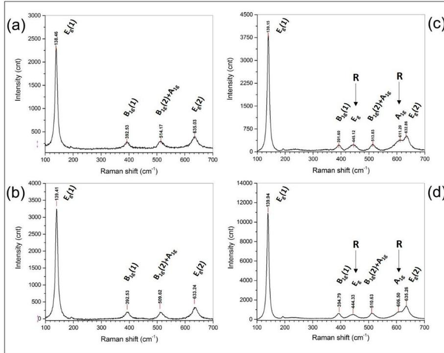
**Figure S3.** Raman spectra of (a) P25-UN; (b) P25-N-HT; (c) P25-F-HT; and (d) P25-F&N-HT. The bands corresponding to rutile were annotated with the letter R.
