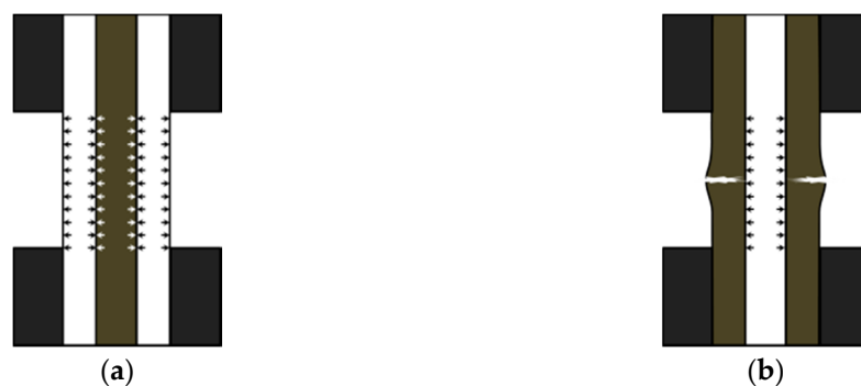
Figure 5. Internal stress diagram with (a) Carbon fiber inside, and (b) Carbon fiber outside under compression.
