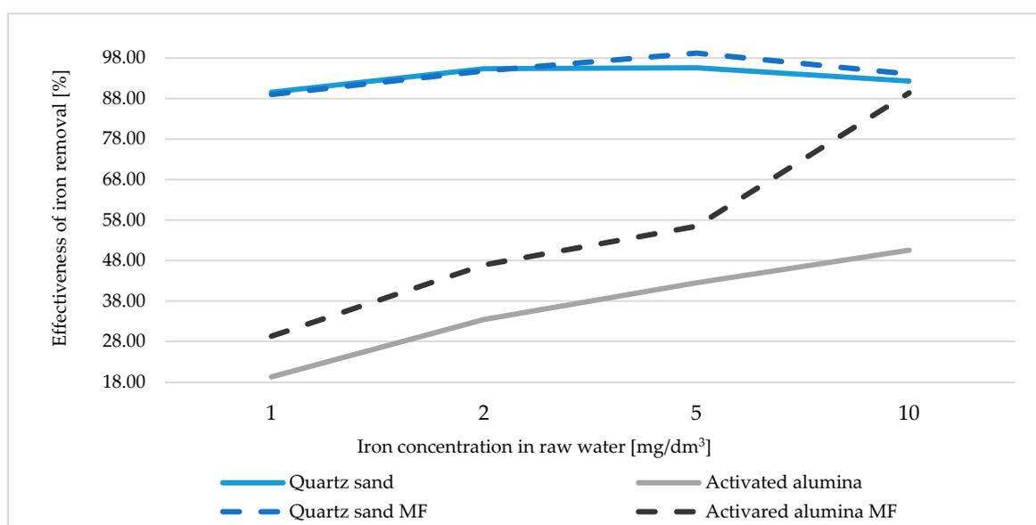
**Figure 1.** Graph of the dependence of the iron removal efficiency on initial concentration in raw water.
