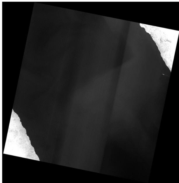
Stray light has been determined to be the cause of the banding issues in TIRS Earth imagery. Unwanted signal from outside the FOV is entering the optical system and adds to the direct line-of-sight signal recorded by the focal plane arrays. The stray light produces a non-uniform signal across the arrays depending on the strength of the source from outside the FOV and also on the view geometry of the detector. The band11 detectors have shown a greater magnitude of the stray light effects than the
