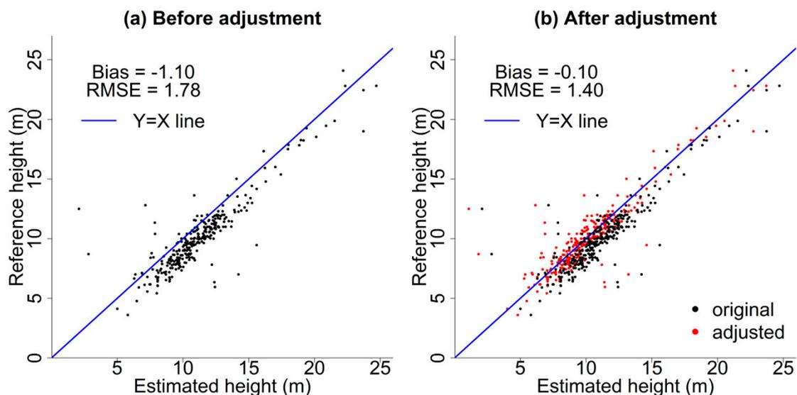
**Figure 11.** The comparisons between (a) original height estimation from the HPC-based MAXI surface and (b) adjusted height estimation with simple subtraction refine process using the radius = 3 m and intensity range = 0.05.
