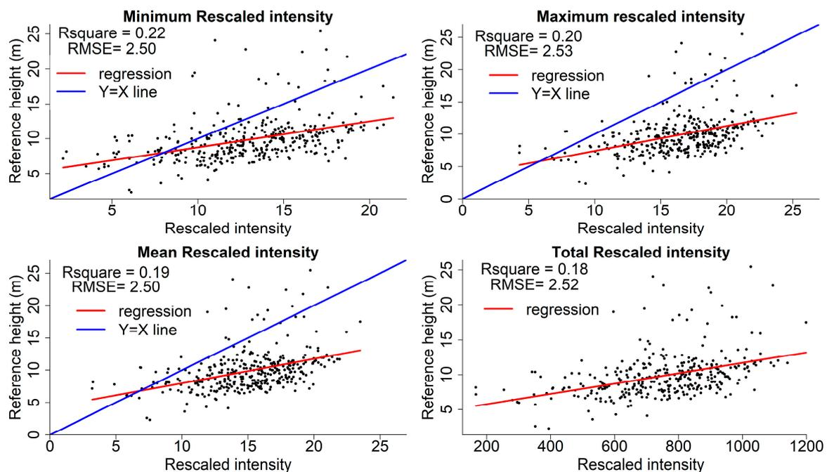
**Figure 10.** The linear relationship between reference tree height and mean rescaled intensity (minimum, maximum, mean and total rescaled intensities) within the 2.5 m buffer of the waveform intensity surface (WIS, 0.5 m resolution).
