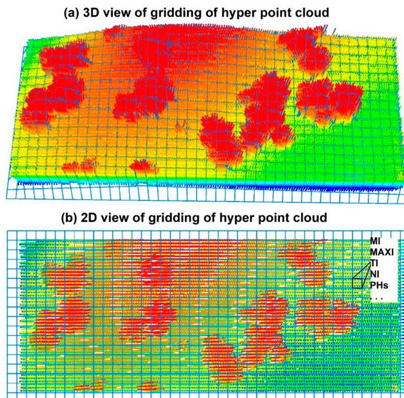
**Figure 4.** The gridding of the hyper point cloud (HPC). (a) 3D view of the HPC with grid-nets. (b) Derivation of variables such as the mean intensity (MI), the maximum intensity (MAXI), the total intensity (TI), the number of intensities (NI) and multiple percentile heights (PHs) at the grid cell level with the gridding procedure from the 2D perspective.
