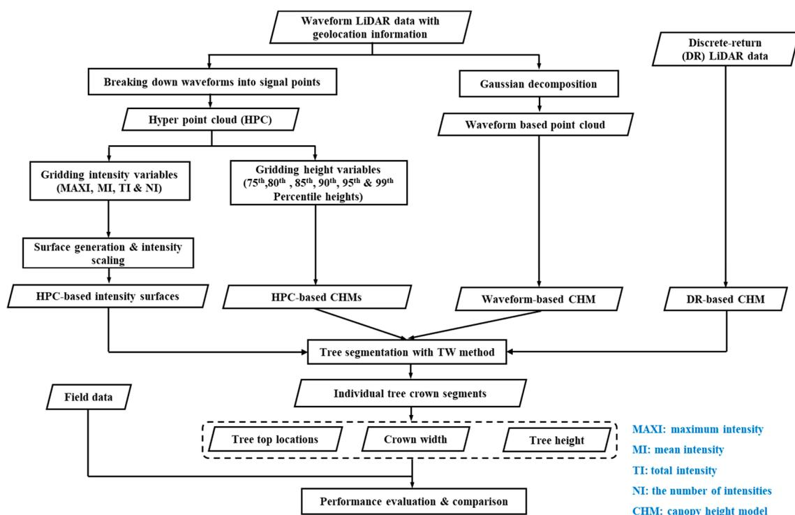
**Figure 2.** The flowchart of utilizing the hyper point cloud to extract tree attributes.
