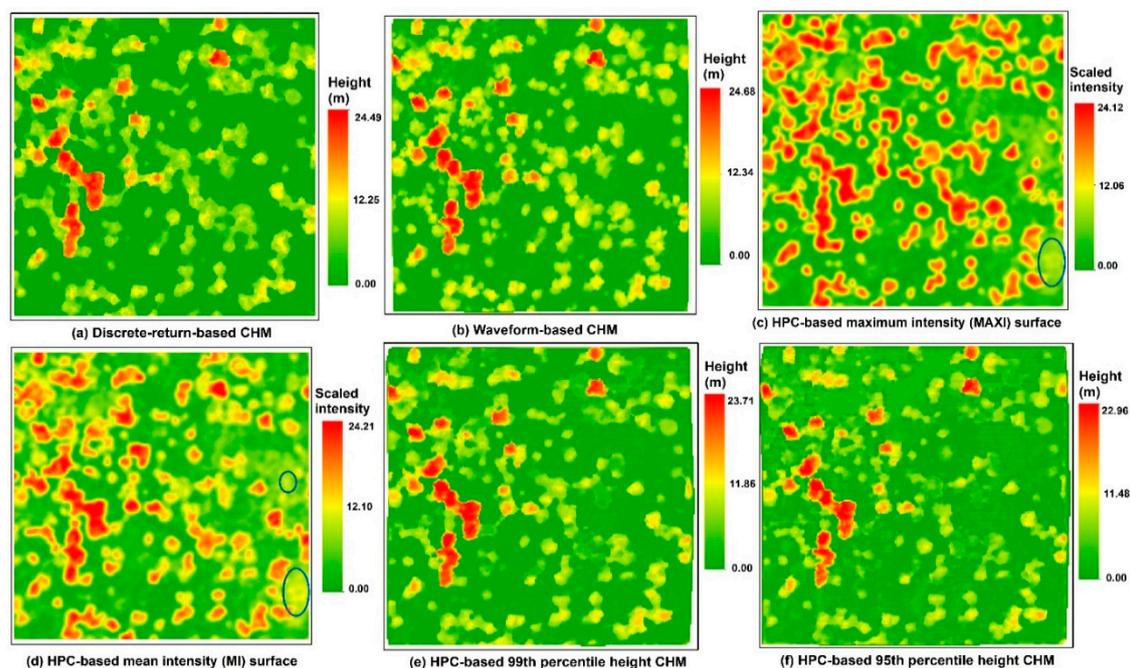
**Figure 7.** Comparisons of the (a) DR-based CHM, (b) waveform-based CHM, (c) HPC-based maximum intensity (MAXI) surface, (d) HPC-based mean intensity (MAXI) surface, (e) HPC-based 99th PH CHM, and (f) HPC-based 95th PH CHM over a subset region.
