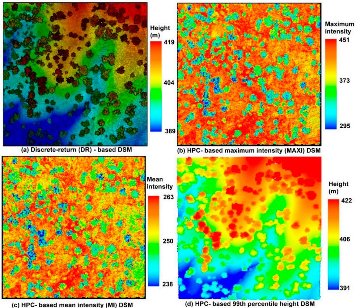
**Figure 5.** Preliminary results of (a) the discrete-return (DR)-based digital surface model (DSM) and (b) the HPC-based MAXI DSM, (c) HPC-based MI DSM, and (d) HPC-based 99th percentile height (PH) DSM from the hyper point cloud (HPC).
