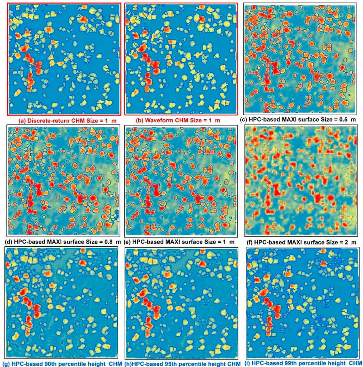
**Figure 9.** Tree crown segmentation results using (a) discrete-return, (b) waveform-based CHMs (red), HPC-based intensity surfaces with different grid cell sizes (c) 0.5 m, (d) 0.8 m, (e) 1 m, and (f) 2 m (black), (g) HPC-based 90th PH, (h) 95th PH, and (i) 99th PH CHM (blue) over the subset region.
