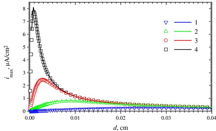
**Figure 2.** The dependence of the maximal biosensor current  $i_{\max}$  on the thickness  $d$  of the enzyme membrane at four maximal enzymatic rates  $V_{\max}$ :  $10^{-9}$  (1),  $10^{-8}$  (2),  $10^{-7}$  (3) and  $10^{-6}$  (4)  $\text{mol}/\text{cm}^3\text{s}$ ,  $S_0 = 2 \times 10^{-8} \text{ mol}/\text{cm}^3$ . Symbols are numerical solutions, while lines are analytical ones (formula 12).
