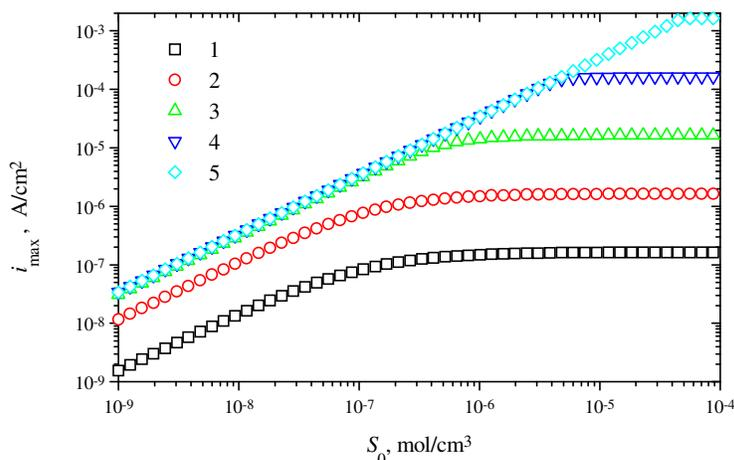
**Figure 7.** The dependence of the maximal biosensor current  $i_{\max}$  on the substrate concentration  $S_0$  at five maximal enzymatic rates  $V_{\max}$ :  $10^{-10}$  (1),  $10^{-9}$  (2),  $10^{-8}$  (3),  $10^{-7}$  (4) and  $10^{-6}$  (5) mol/cm<sup>3</sup>s,  $d = d_8(10^{-8}, 10^{-6}, 2 \times 10^{-8}) = 0.017$  cm, calculated by formula (18) accepting  $\delta = 0.1$ .
