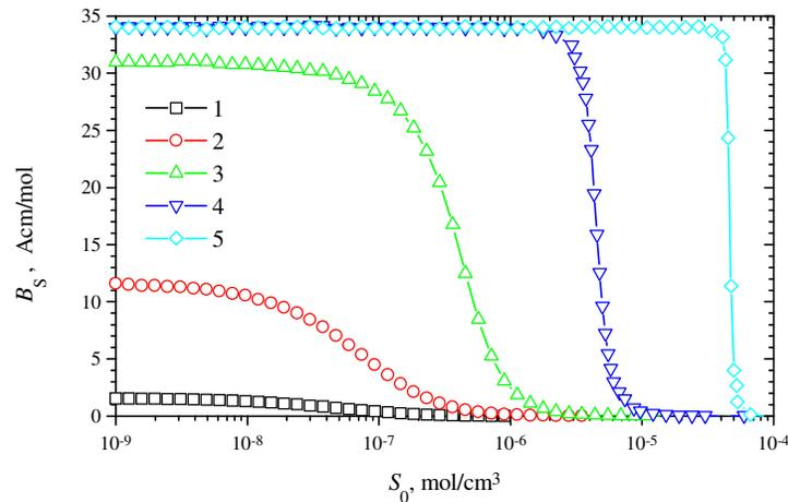
**Figure 8.** The dependence of the biosensor sensitivity  $B_S$  (formula 20) on the substrate concentration  $S_0$  at five maximal enzymatic rates  $V_{\max}$ :  $10^{-10}$  (1),  $10^{-9}$  (2),  $10^{-8}$  (3),  $10^{-7}$  (4) and  $10^{-6}$  (5)  $\text{mol}/\text{cm}^3\text{s}$ . Other parameters are the same as in Fig. 7.
