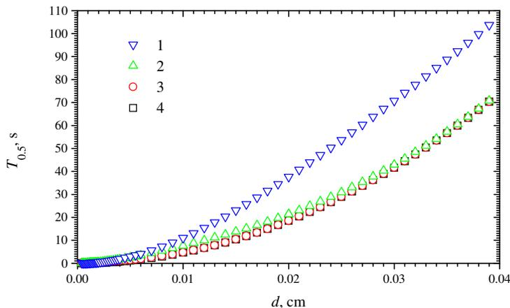
**Figure 3.** The dependence of the half time  $T_{0.5}$  of the maximal biosensor current on the membrane thickness  $d$  at four maximal enzymatic rates  $V_{\max}$ :  $10^{-9}$  (1),  $10^{-8}$  (2),  $10^{-7}$  (3) and  $10^{-6}$  (4)  $\text{mol}/\text{cm}^3\text{s}$ ,  $S_0 = 2 \times 10^{-8} \text{ mol}/\text{cm}^3$ .
