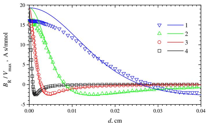
**Figure 9.** The biosensor resistance  $B_R$  (formula 21), normalised with the maximal enzymatic rate  $V_{\max}$ , versus the membrane thickness  $d$ . Symbols are numerical solutions, while lines are analytical ones (formula 14). All parameters are the same as in Fig 2.
