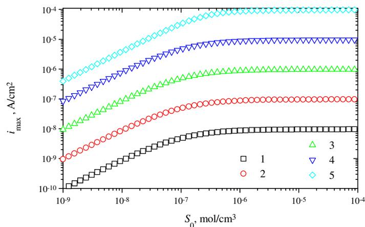
**Figure 6.** The dependence of the maximal biosensor current  $i_{\max}$  on the substrate concentration  $S_0$  at five maximal enzymatic rates  $V_{\max}$ :  $10^{-10}$  (1),  $10^{-9}$  (2),  $10^{-8}$  (3),  $10^{-7}$  (4) and  $10^{-6}$  (5) mol/cm<sup>3</sup>s,  $d = 0.001$  cm.
