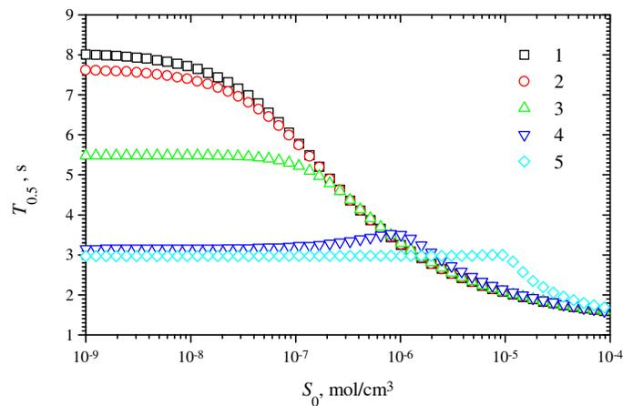
**Figure 5.** The dependence of halftime  $T_{0.5}$  of the maximal biosensor current on the substrate concentration  $S_0$  at five maximal enzymatic rates  $V_{\max}$ :  $10^{-10}$  (1),  $10^{-9}$  (2),  $10^{-8}$  (3),  $10^{-7}$  (4) and  $10^{-6}$  (5) mol/cm<sup>3</sup>s, other parameters are the same as in Fig. 4.
