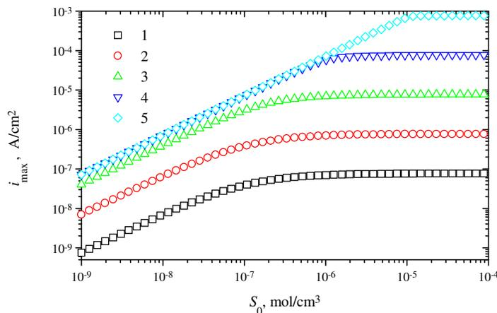
**Figure 4.** The dependence of the maximal biosensor current  $i_{\max}$  on the substrate concentration  $S_0$  at five maximal enzymatic rates  $V_{\max}$ :  $10^{-10}$  (1),  $10^{-9}$  (2),  $10^{-8}$  (3),  $10^{-7}$  (4) and  $10^{-6}$  (5)  $\text{mol}/\text{cm}^3\text{s}$ ,  $d = d_\delta(10^{-7}, 10^{-6}, 2 \times 10^{-8}) = 0.008 \text{ cm}$ , calculated by formula (18) assuming  $\delta = 0.02$ .
