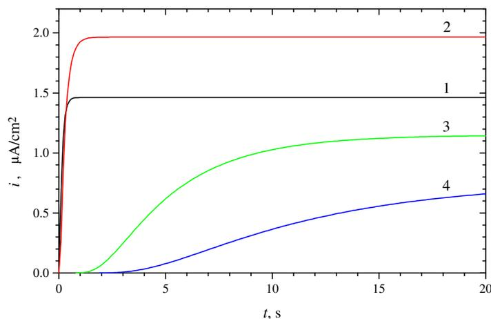
**Figure 1.** The dynamics of the biosensor current  $i$  at the maximal enzymatic rate  $V_{\max} = 10^{-7} \text{ mol/cm}^3\text{s}$  and four membrane thickness  $d$ : 0.001 (1), 0.0015 (2), 0.01 (3), 0.015 (4) cm,  $S_0 = 2 \times 10^{-8} \text{ mol/cm}^3$ .
