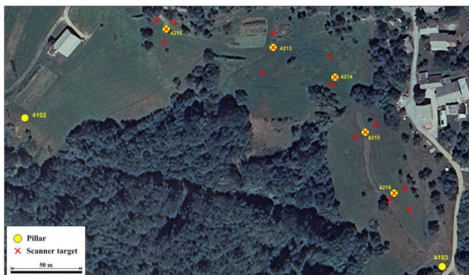
Figure 3. The geodetic network designed near the object of the study.
