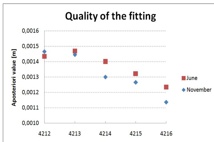
Besides, the spatial distribution of residuals suggests that the selection of the scanner locations, as shown in Figure 4, actually compensated for the considerable errors of individual scans in the scanning direction, which is one of the downsides of the time-of-flight type scanners also employed in our
