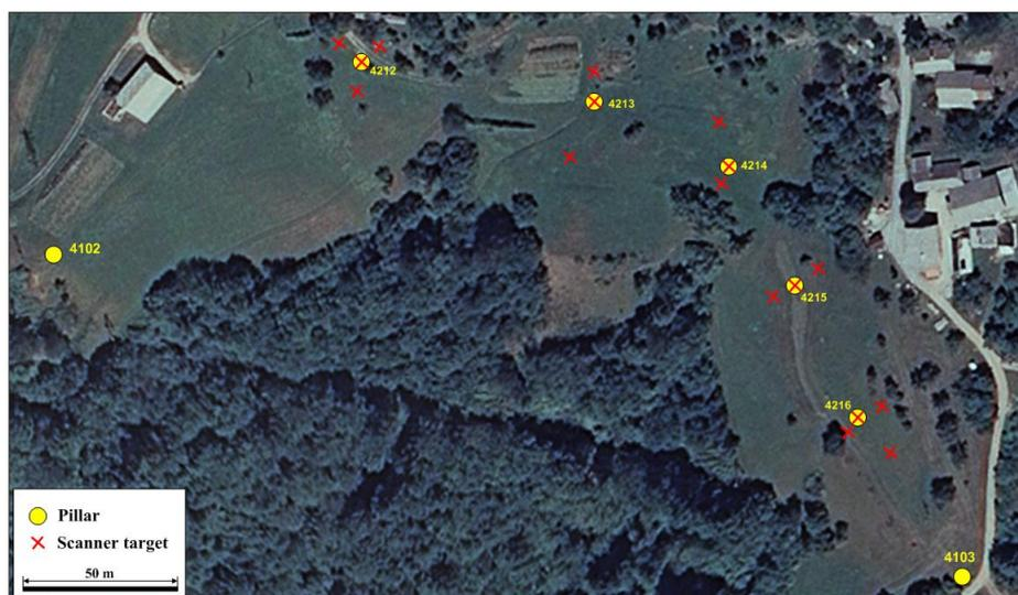
Apart from the observation pillars (Figure 3), the scanner targets were placed onto the tripods. In the process of tacheometric measurements, also the reference pillars 4102 and 4103 were included which made it possible to compare the adjusted base distance 4102–4103 with the GNSS data.
