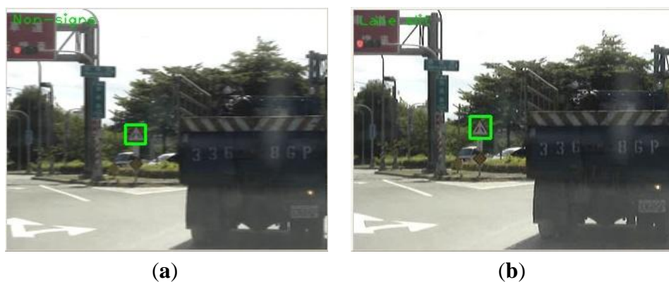
Figure 14. Blurred image may cause error: (a) the detection result of the 41st frame of video sequence #08; (b) the next frame, which can be recognized correctly.
