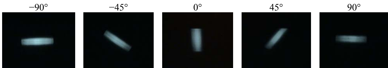
Figure 12. Shape of the laser beam at different scanning angles.
