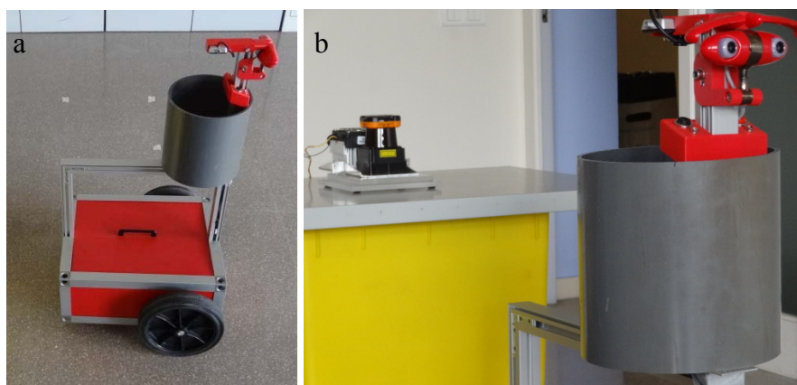
Figure 15. Images of the mobile robot with a circular marker attached (a) and the laser scanner (b).
