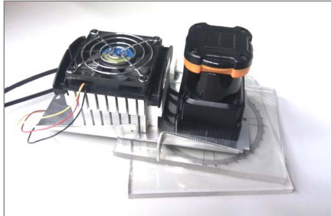
Figure 2. Laser sensor and additional cooler on a rotating structure.
