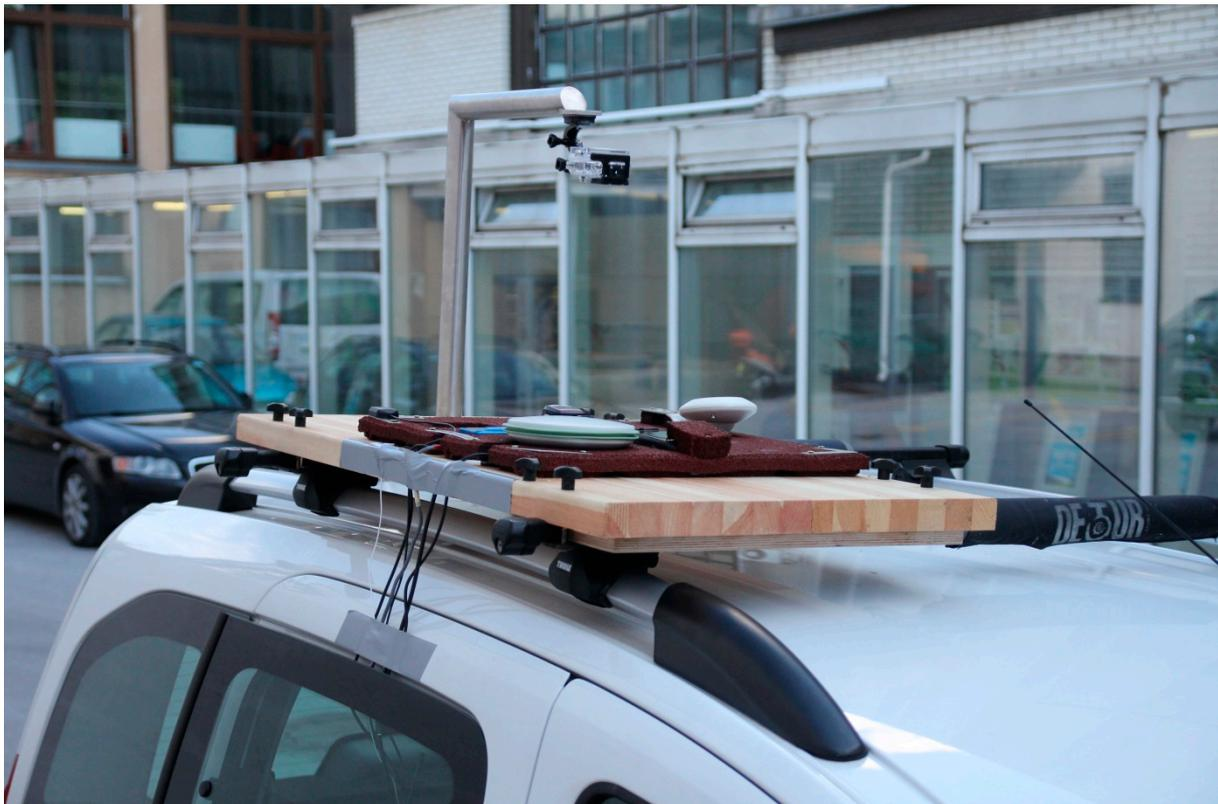
Five different GNSS devices ranging from a simple consumer product to high-end high-frequency real time kinematics (RTK) GNSS devices have been used in the study:
