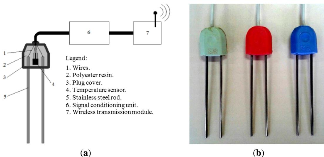
**Figure 1.** (a) Probe for measuring water content and apparent electrical conductivity of soil; (b) Probes for measuring temperature, electrical conductivity and relative dielectric constant.
