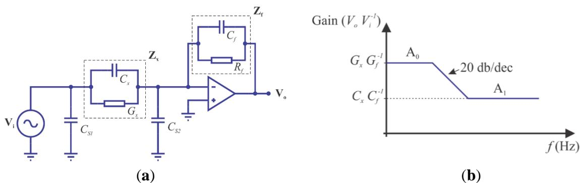
**Figure 2.** (a) Auto-balancing bridge circuit and frequency domain response (b).
