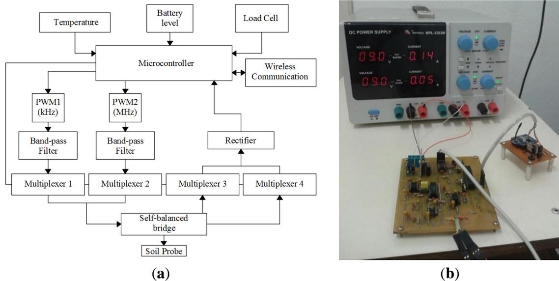
**Figure 3.** (a) Signal-conditioning unit circuit diagram; (b) Signal-conditioning unit implemented circuit.
