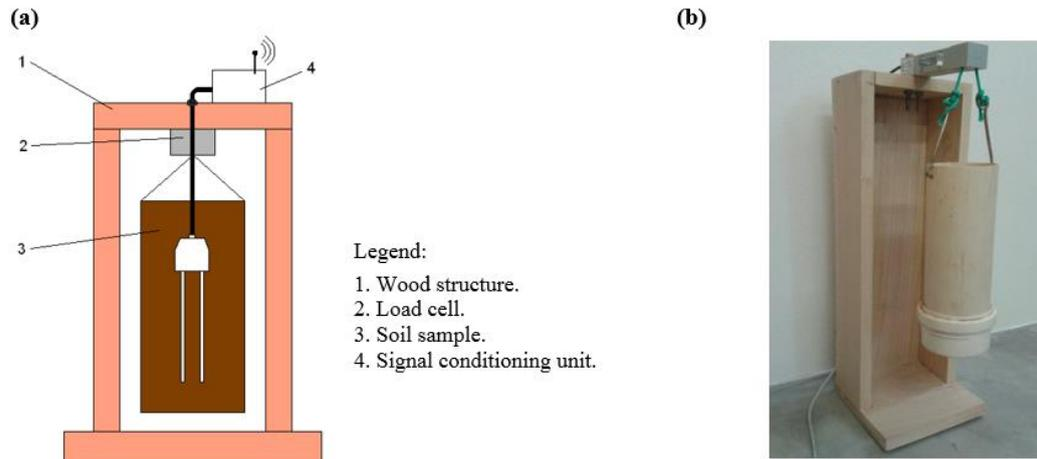
**Figure 4.** (a) Scheme support structure of the soil samples; (b) Structure of weighing the soil samples.
