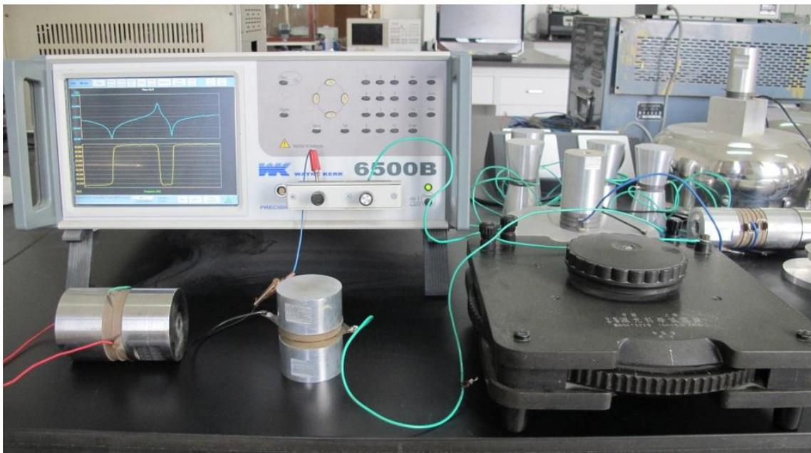
**Figure 12.** Experimental set-up for the measurement of the frequency response.
