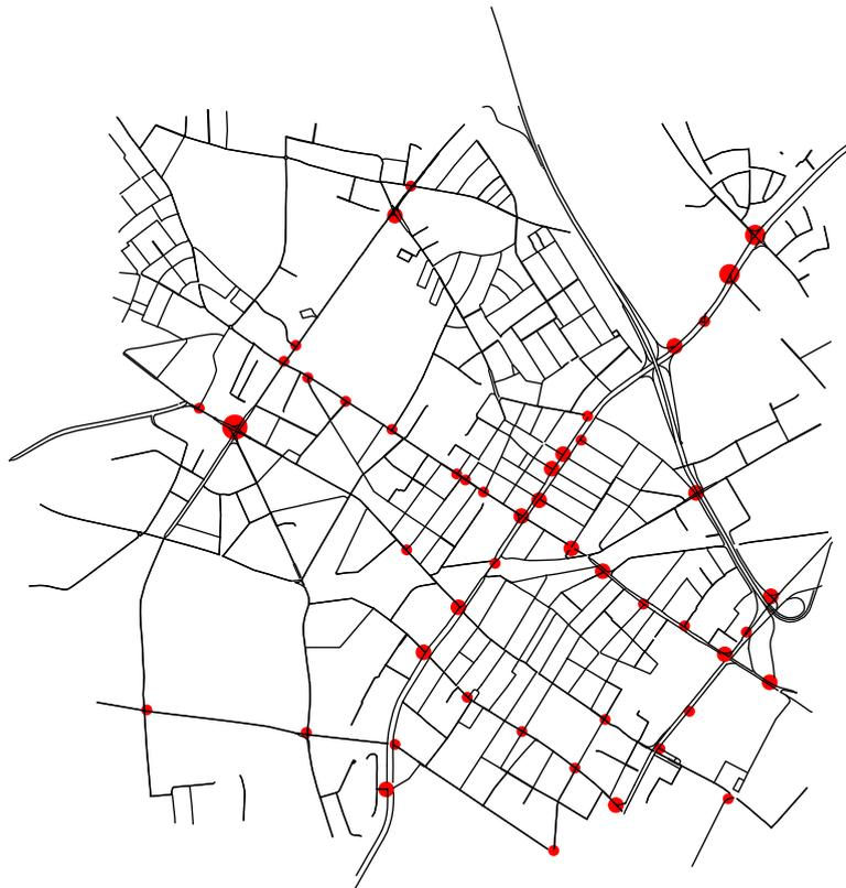
**Figure 5.** Representation of network edges (black lines) and intersection agents (red dots).
