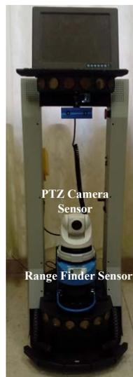
**Figure 1.** The PeopleBot mobile robot platform, where several sensors are attached to the robot, e.g., pan-tilt-zoom (PTZ) camera, laser range finder, sonars, stereo camera, etc.
