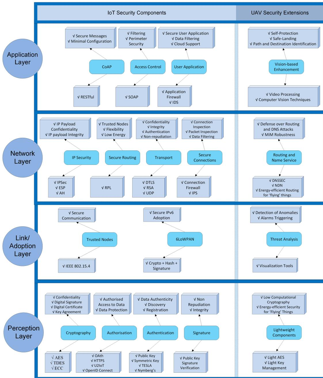
Figure 2. IoT security layers with UAV extensions.
