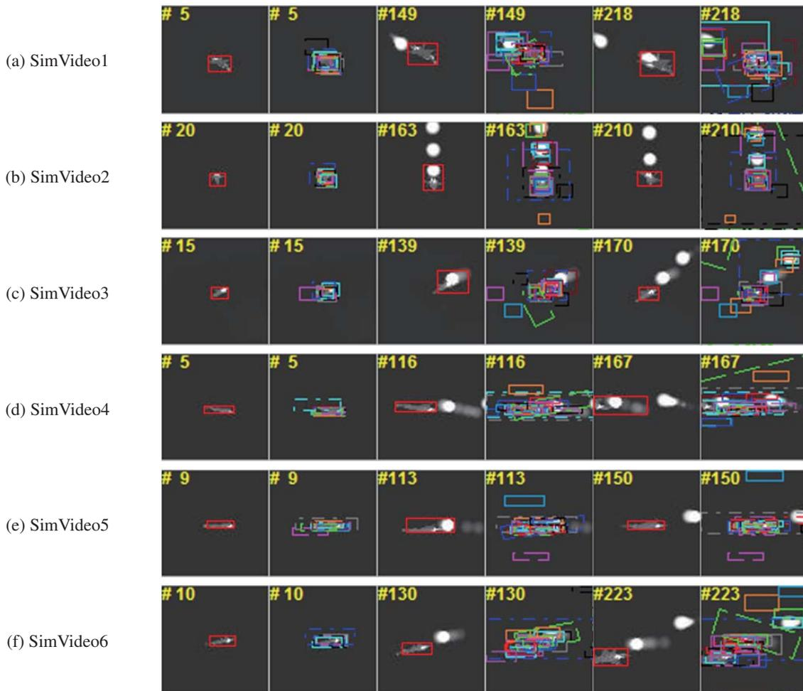
**Figure 19.** Tracking results of simulated infrared sequences. Our tracker's results are drawn with a red rectangle for clarity.
