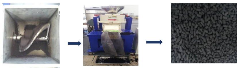
Figure 1. Processing diagram of biochar pellet with different pig compost ratios.
