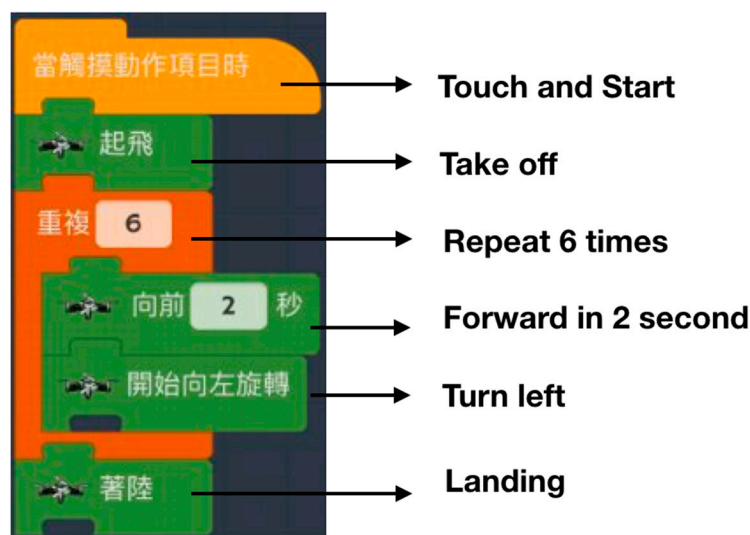
Figure 4. Drone programming example (flying in a large circle).
