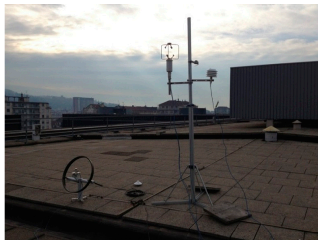
Figure 3. External meteorological station.
