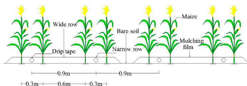
**Figure 3.** Layout of the design of mulched drip irrigation in this study. The unit of the numbers is m.
