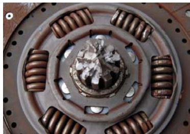
Figure 1: A broken shaft in the clutch
